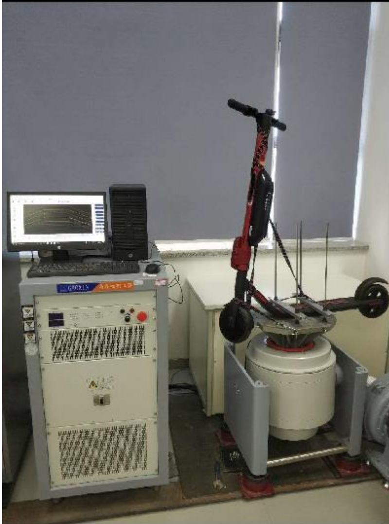
Image on the left: A device undergoing a 'vibration test' (photo credit: TUV Rheinland)
