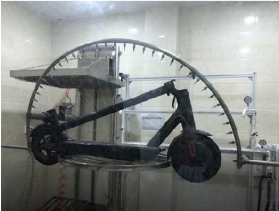
Image on the left: A device undergoing an 'IPX4 test' (photo credit: SGS Testing & Control Services)
