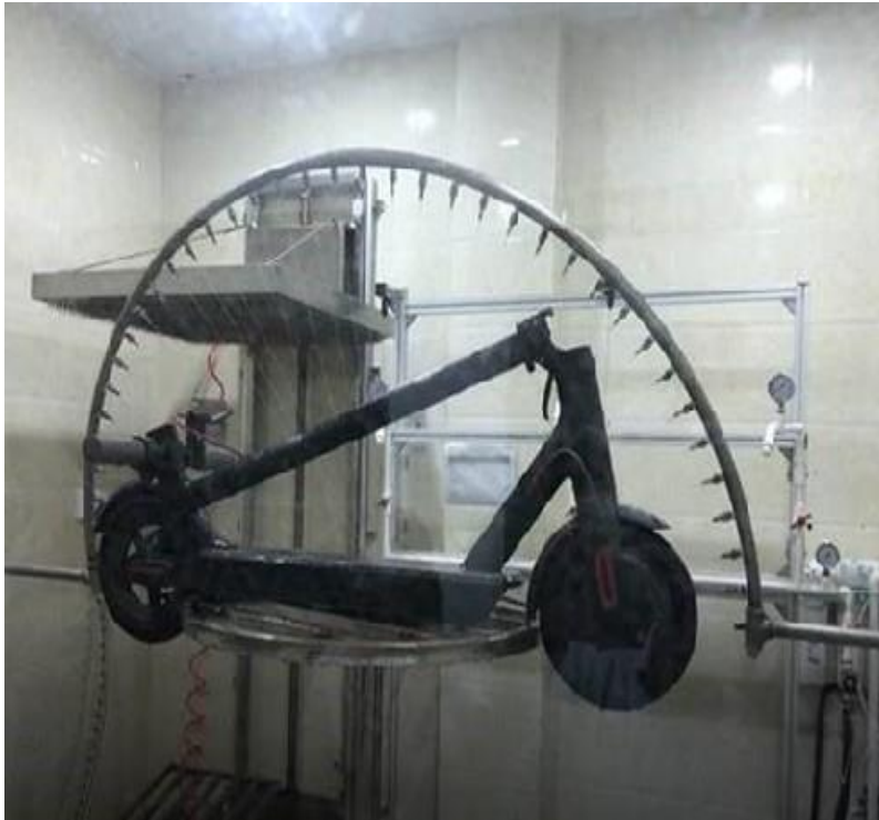
Image on the left: A device undergoing an 'IPX4 test' (photo credit: SGS Testing & Control Services)
