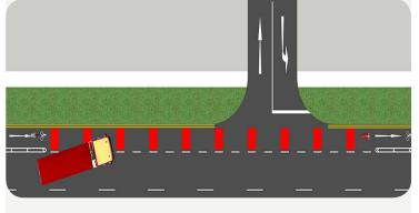
Red Transverse Lines are located **at junctions and before every access** for vehicles to weave and turn into side roads. These lines are also located **after every access** for vehicles turning out into the main carriageway.
