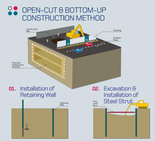
The underground retaining wall is installed before excavation commences. The retaining wall can be a concrete diaphragm wall, a concrete bored pile wall or a steel sheet pile wall; depending on the site condition, soil type and the excavation depth. The soil is excavated to the first strut level. The first level strut is installed before the excavation proceeds further.
