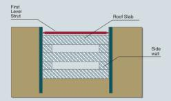
The next level of slab is constructed, followed by the removal of the strut near to that slab level. This process progresses upwards till the roof slab is constructed. 04. Construction of Underground Structure
