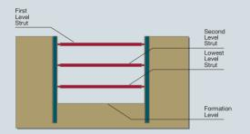
The soil is excavated to the next strut level and the second level strut is installed. It continues till the excavation reaches the final depth or formation level. The number of strut levels depends on the excavation depth.
