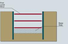
At formation level, the reinforced concrete slab or base slab is constructed, followed by the removal of the lowest level strut and the side walls are constructed.
