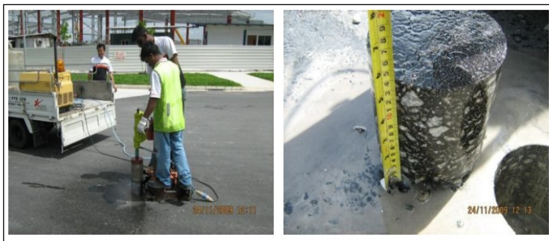
Figure 14.3 Coring of Premix
