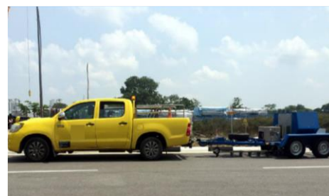
FWD test for structural capacity check
