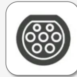
Type 2 Alternating Current (AC Charging)
