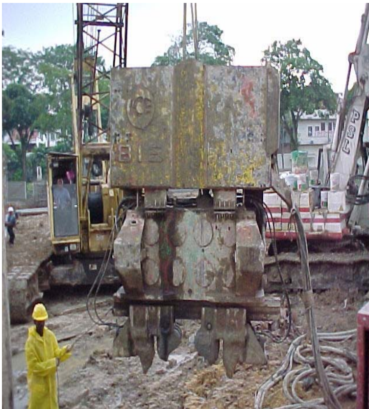
Figure 3-8 View of a vibro-hammer
