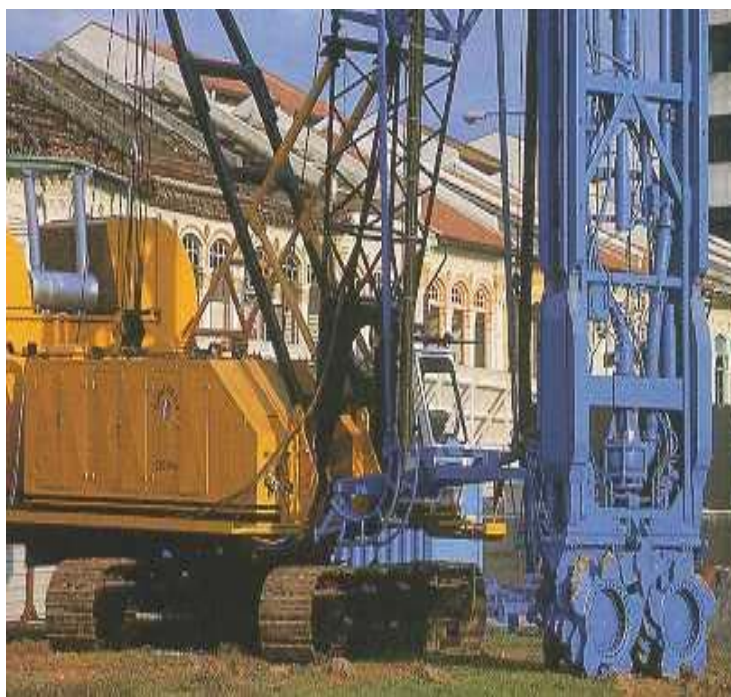
Figure 3-6 View of a hydrofraise machine
