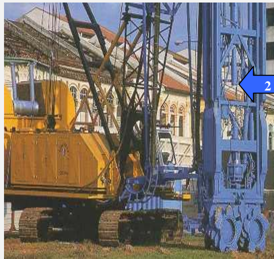
Figure 3-6 View of a hydrofraise machine
