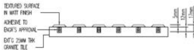
SECTION THRU' TILE (STAINLESS STEEL STUDS)
