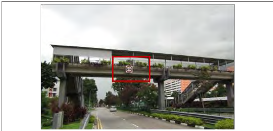
Figure 20: 4.5m Height Restriction Sign Installed Strategically on a POB
