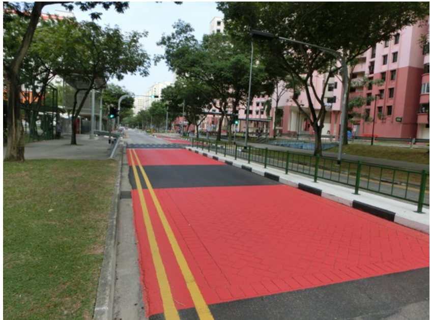
The red textured road surface makes the school zone more noticeable
