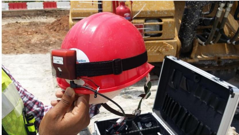
Fig. 1 Helmet sends vibration alerts when the wearer is too close to machinery
