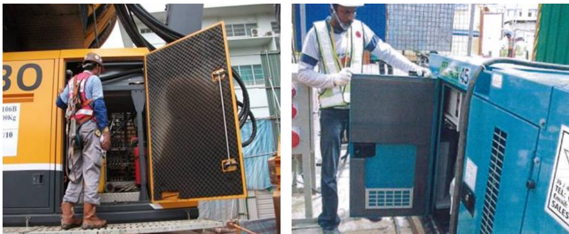
Figure 17: Installation of acoustic material in machineries
