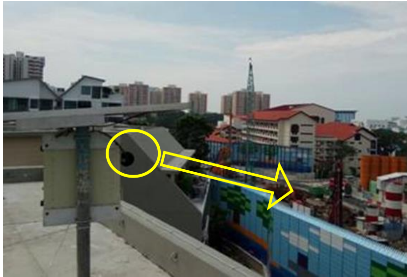
Figure 11: A real-time noise meter installed on the rooftop with microphone facing the construction site
