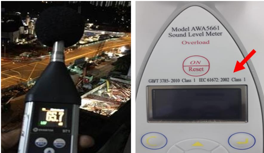
Figure 12: Ad-hoc noise monitoring (left) and Class 1 certified handheld noise meter (right)
