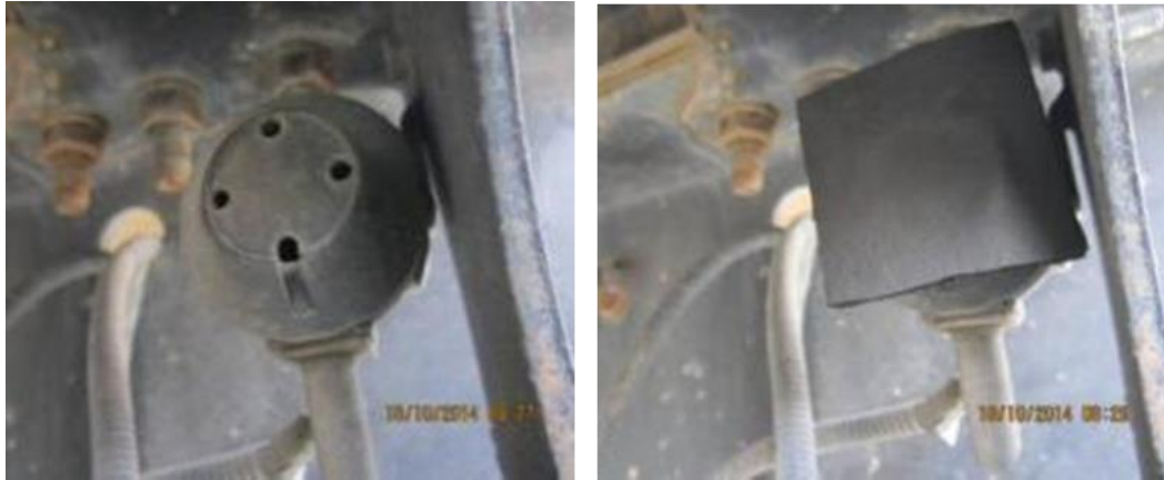
Figure 14: Machine fixed with muffler to minimise beeping noise
