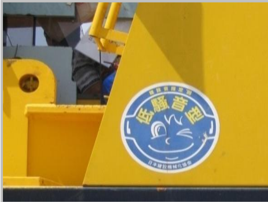
Use of sound-reduced machinery
