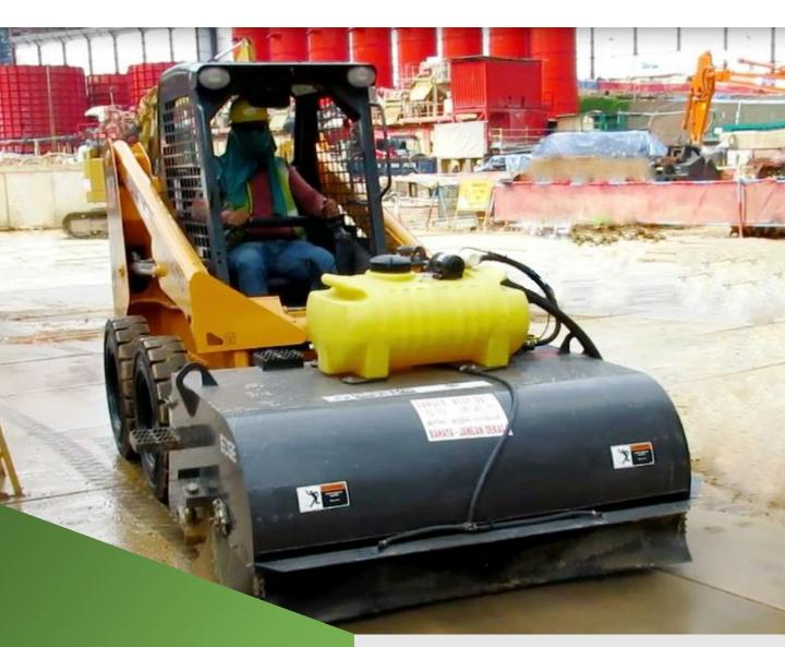
Vacuum Machine with Water Sprayer Provide a vacuum machine with water sprayer to wet vehicular access
