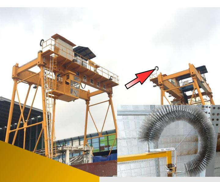
Lightning Dissipation System for Gantry Crane Provide lightning dissipation system for gantry crane.
