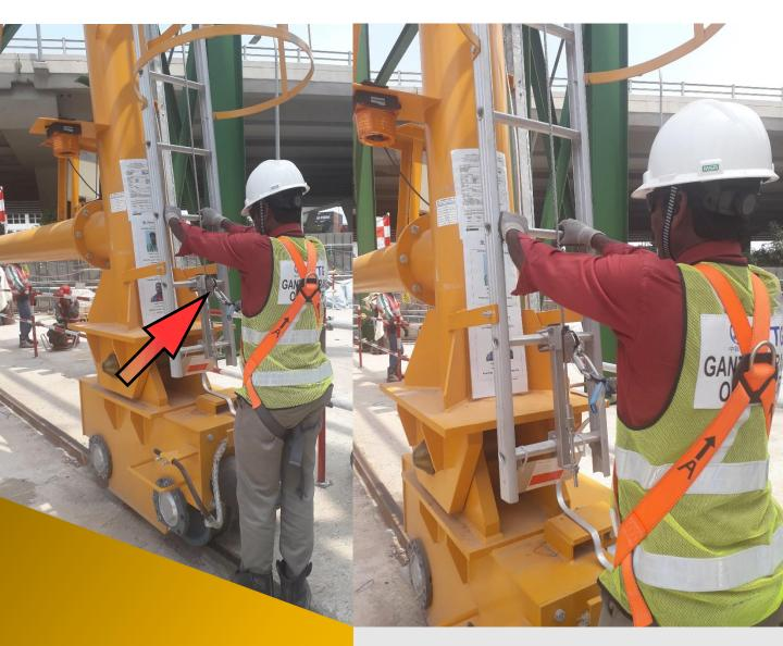
Fall Protection For Gantry Crane Provide fall protection device that eliminates fall from height risks during use of gantry crane access ladder.
