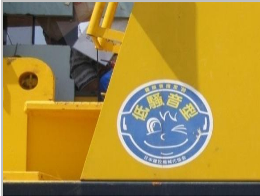
Use of sound-reduced machinery
