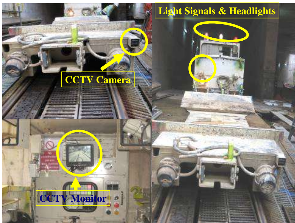
Locomotive equip with camera and monitor for rear view.
