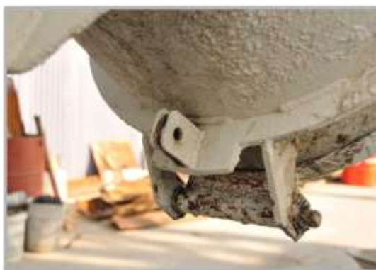
Pin plate at the rear for securing the cover when opened
