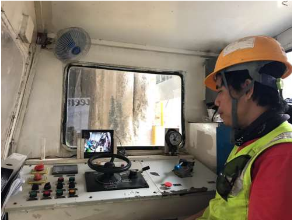
Locomotive equip with camera to monitor rear view
