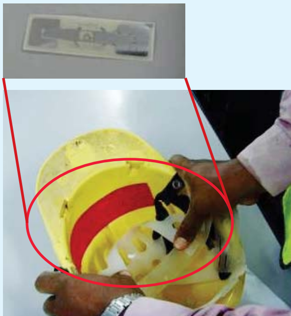
RFID Tag taped inside worker's helmet
