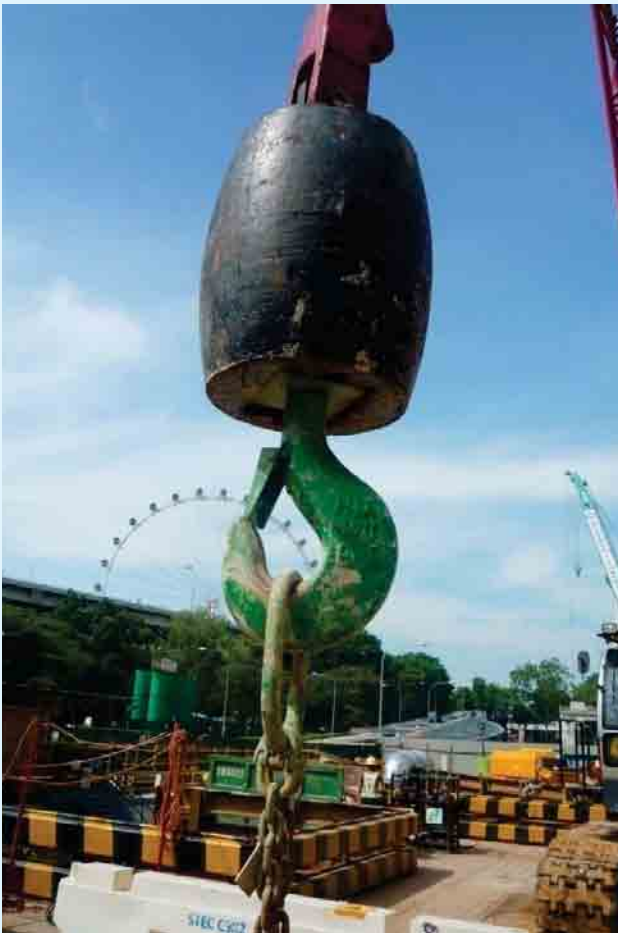
Load hooks with swivel and safety latch
