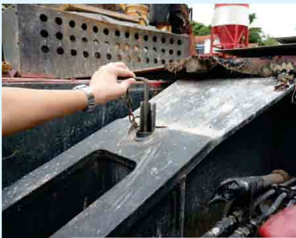
Interlocking device for outriggers
