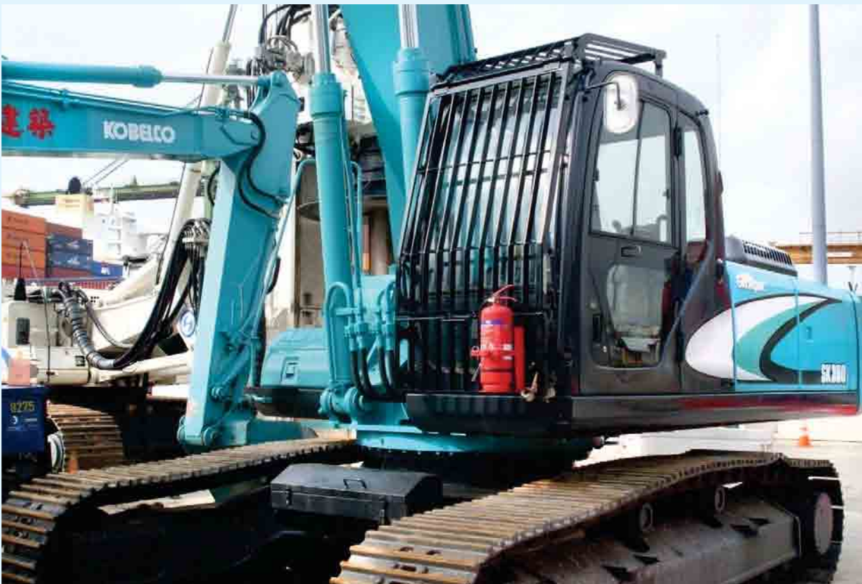
Excavator with reinforced roof
