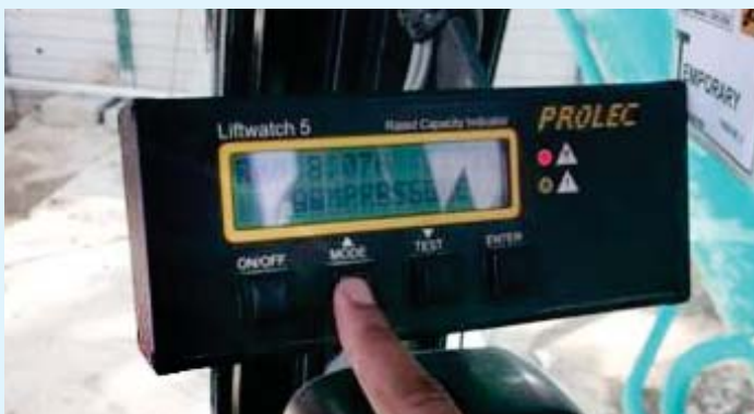
Indicator with working radius and corresponding SWL
