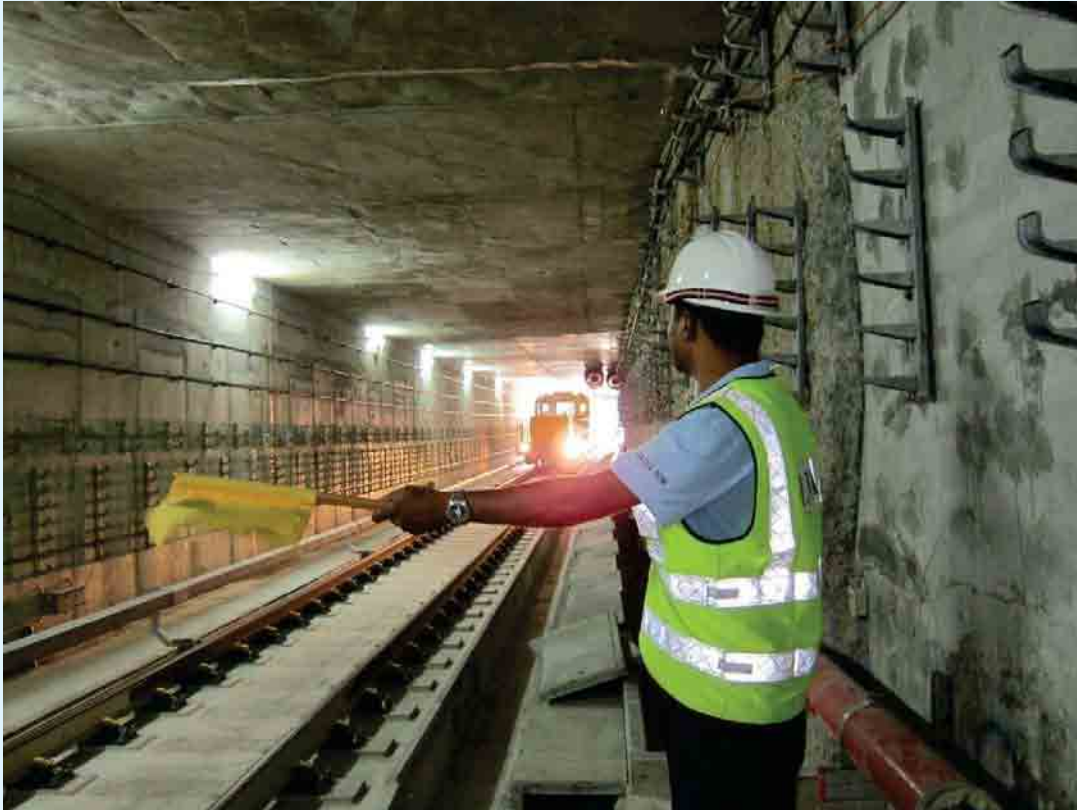
Ground Shunter using coloured flags to direct an approaching train
