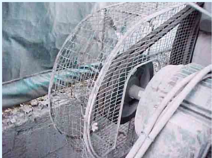
Installing a makeshift guard for rotating flywheel made from wire mesh
