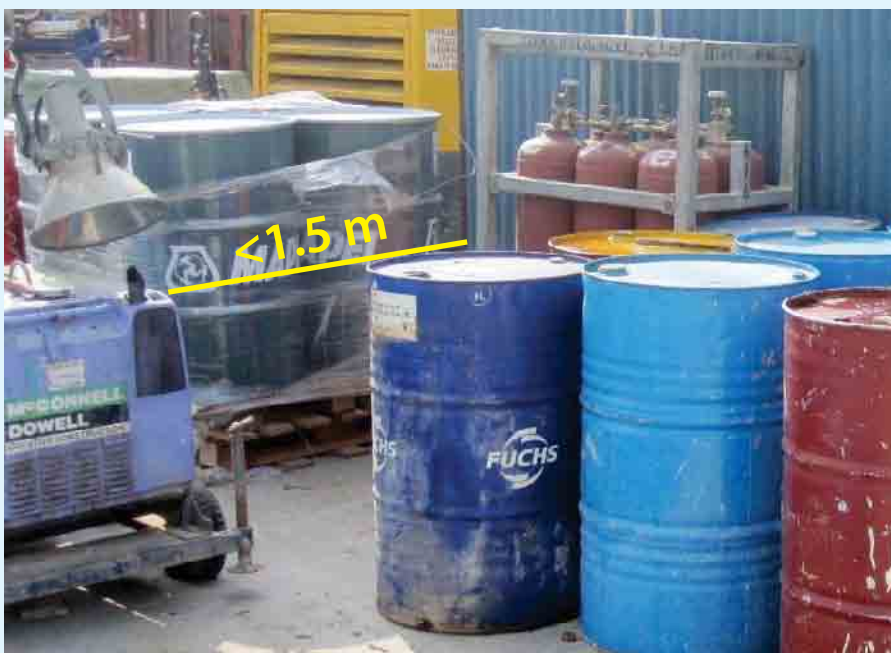
Gas cylinders placed near to radiator
