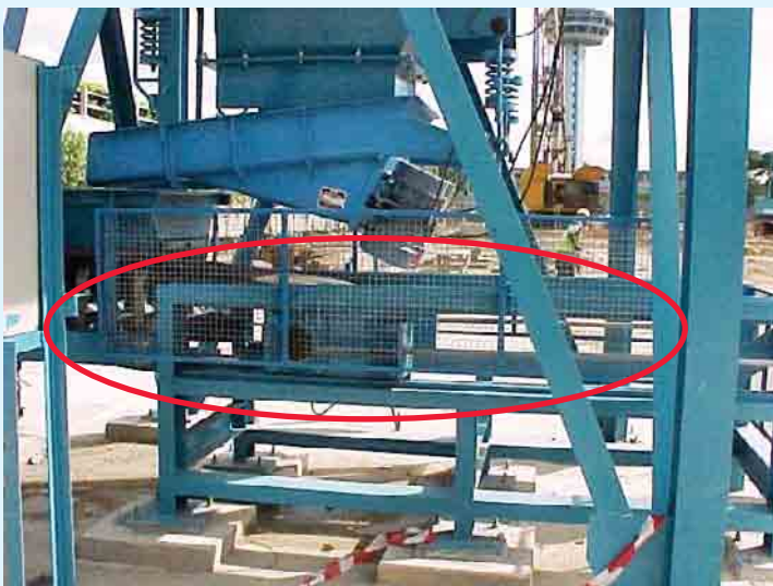
Installing a makeshift guard for rotating flywheel made from wire mesh
