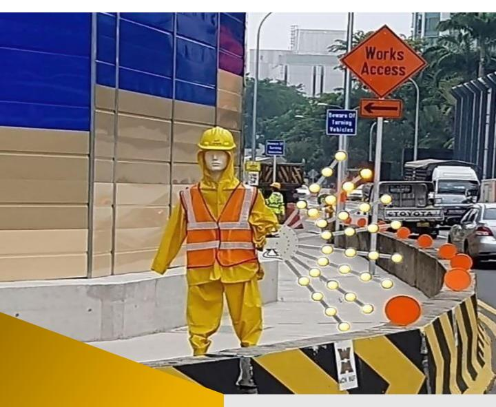
Robotic Traffic Marshal Deploy robotic traffic marshal to guide traffic
