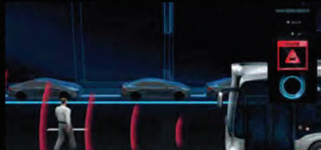
Active Brake Assist: This unique feature automatically initiates a braking manoeuvre with partial braking upon threat of collision.
