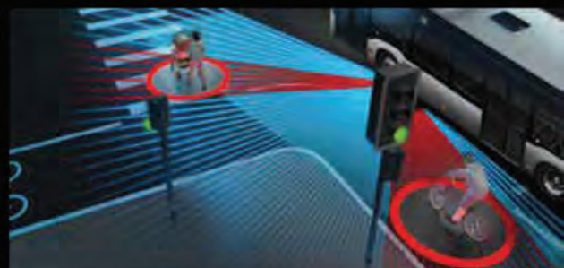
Sideguard Assist: Flashing LED lamps and driver's seat vibrations alert drivers to dangers of collision with stationary or moving objects.
