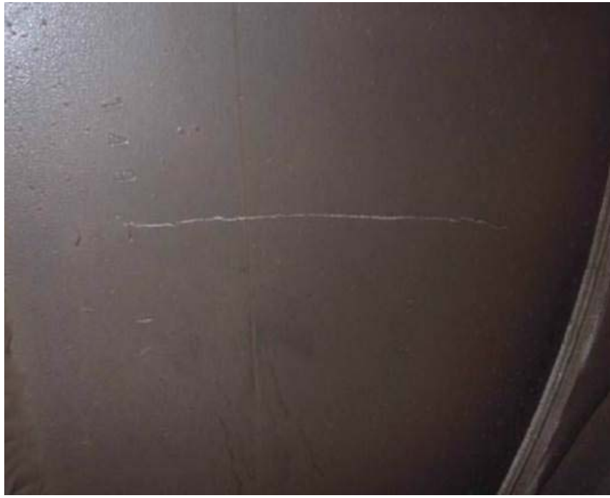
Hairline crack on train bolster – 142mm in length
