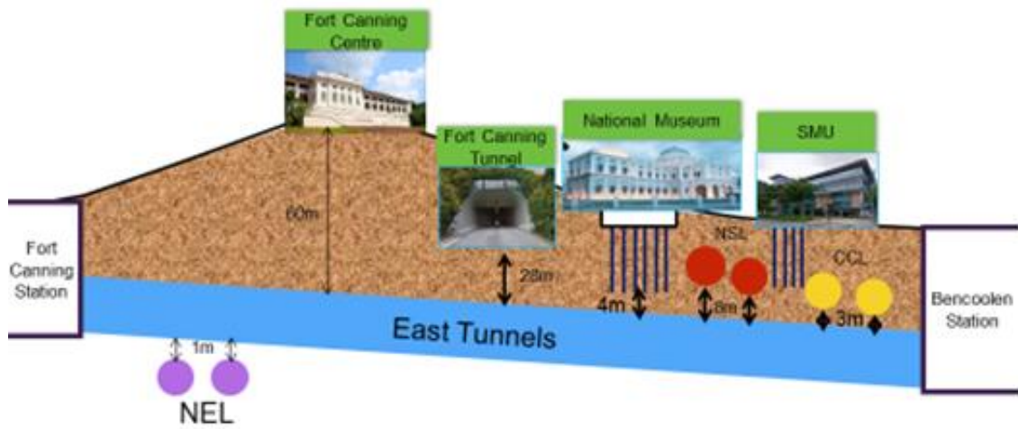
Picture C: Construction of Fort Canning Station and Tunnels in Singapore – Challenges of East Tunnel and its close proximity to other tunnels and national monuments
