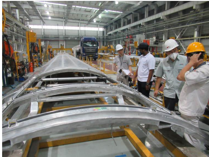
Figure 2: Inspection of train carbody parts
