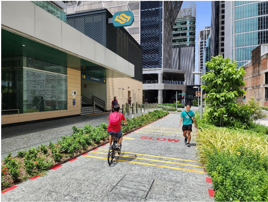
Shenton Way MRT, with dashed red lines on new grey tiled pavement, to demarcate shared walking / cycling path
