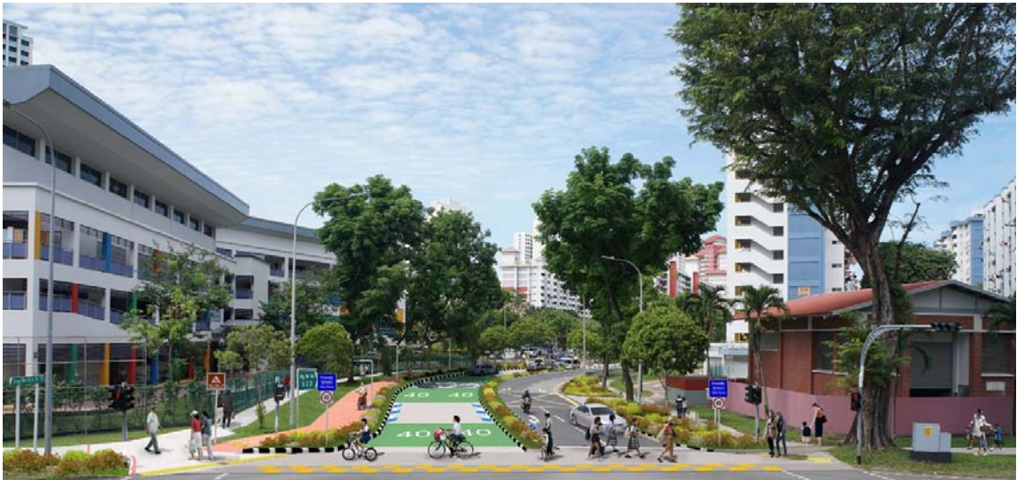
Signs, 3D road markings and coloured road surfaces to signal entry into Friendly Streets
