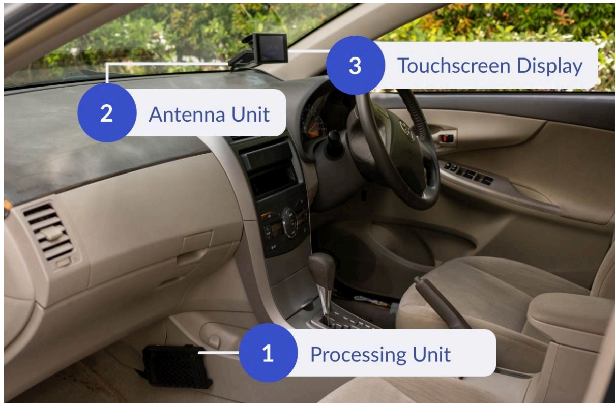
OBU with all three pieces installed in their default positions
