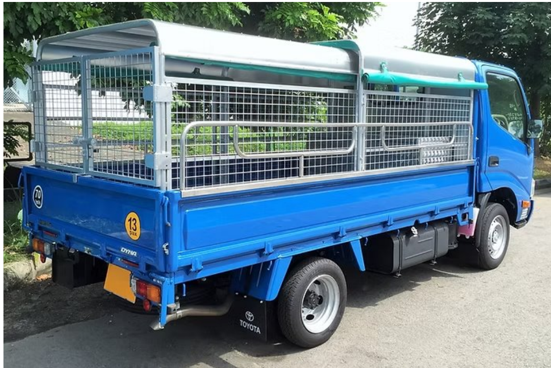
Example of caged lorry decks
