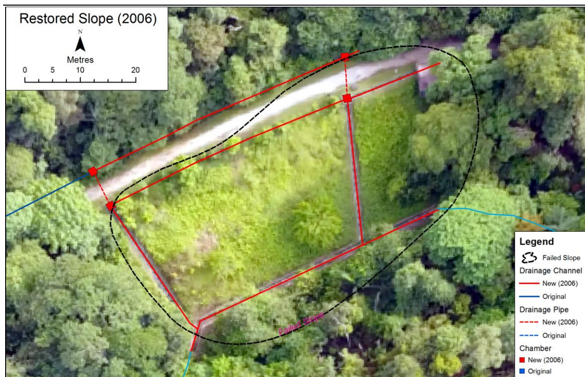
Figure A.4: Repaired Slope and Installed Drainage Infrastructure
