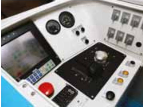
⏏ (Top) The control panel on board the train allows a driver to take over in case of an emergency. (Bottom) Celebrating the arrival of the first Circle Line train.
