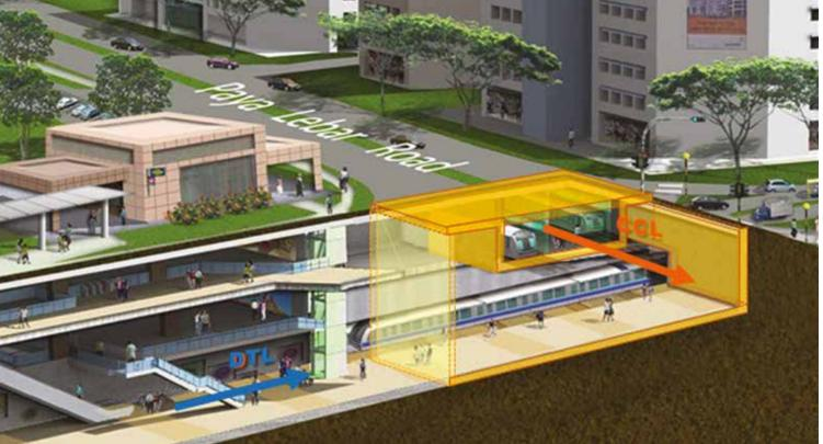
When the contractor for the DTL MacPherson station came on board, it dismantled part of the box's slabs and walls to build new escalators and staircases. The space now provides a seamless connection between the Circle Line and DTL.
