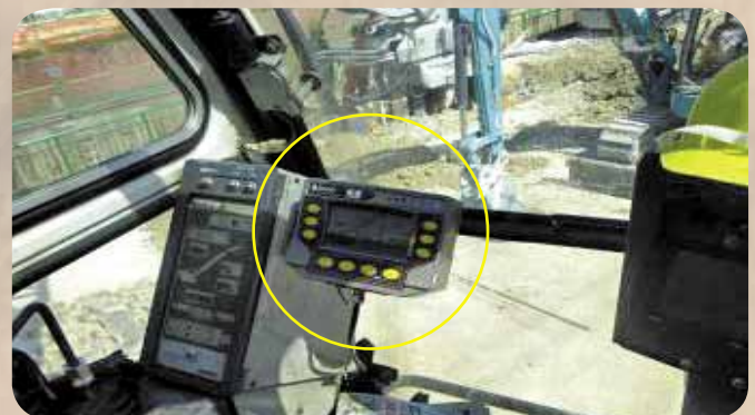
Figure 3: Data logger installed in crane
