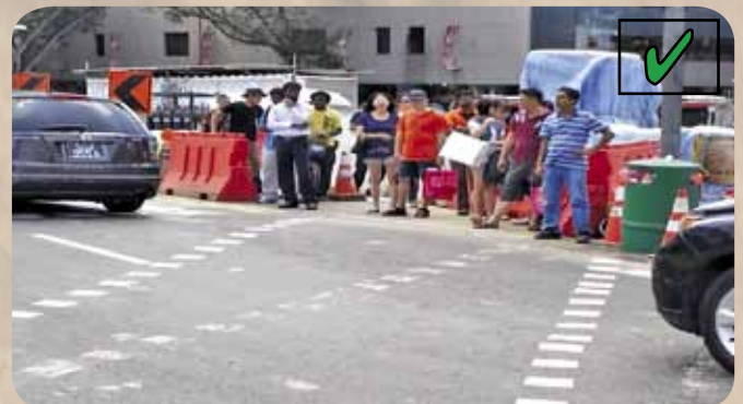
Figure 2b: Aligned pedestrian crossing path with waiting area
