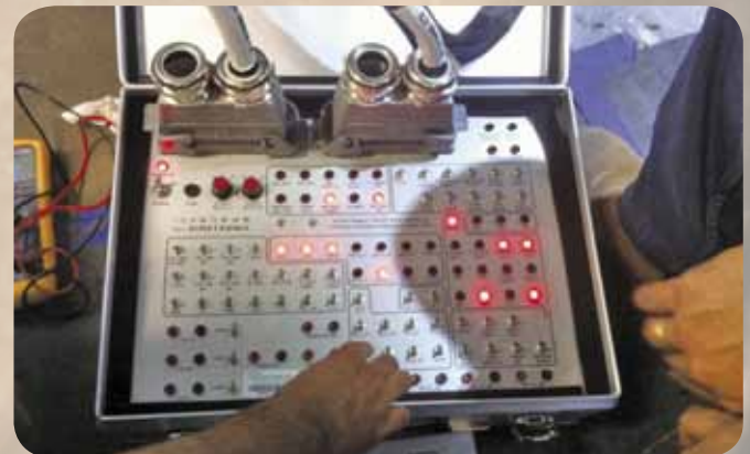
Figure 5: Static Routine Test of the Trainborne Signalling Equipment using simulator for rolling stock inputs & outputs
