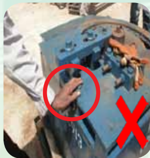
Figure 6: Do not place hands in the path of moving parts at all times
