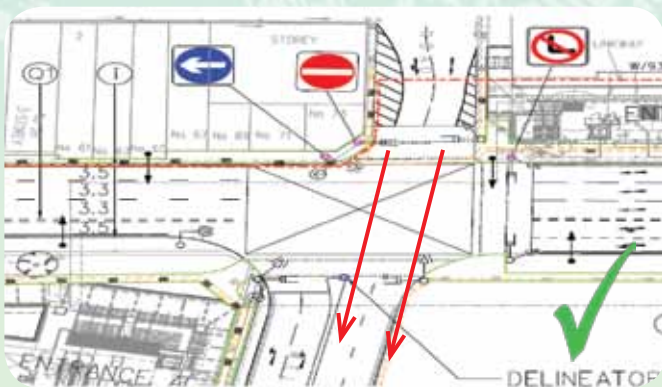
Figure 1b: In order to improve the alignment, chevron marking has been added to guide motorists across the junction
