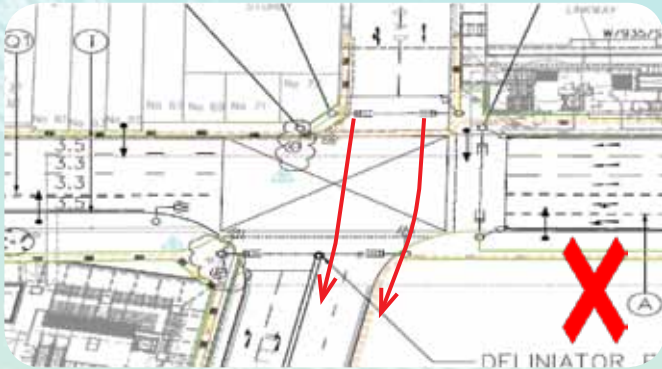
Figure 1a: The approaching lanes do not align with the receiving lanes at the junction
