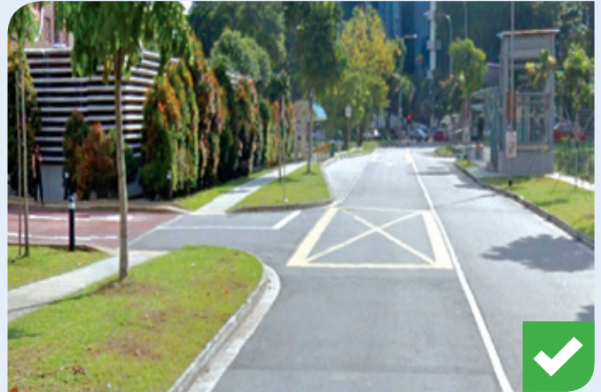
Figure 3: Vent shaft positioned away from corner of side road access to ensure adequate visibility of oncoming vehicles
