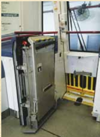
Figure 6: Detrainment stairs stowed to the side in a train-car
