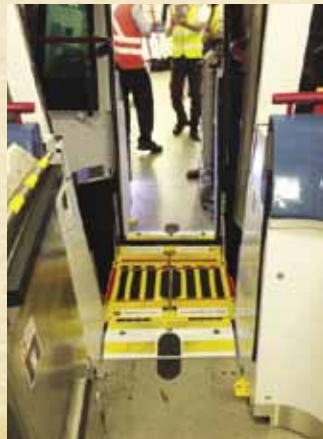
Figure 7: Clear passageway for access to gangway in car-to-car detrainment
