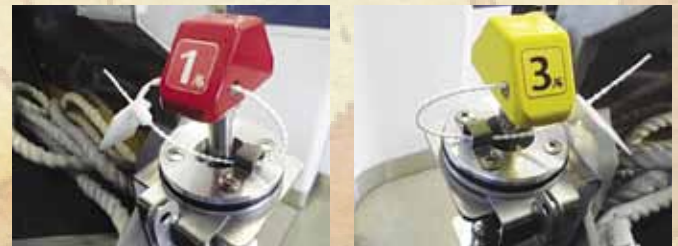
Figure 9: Pictures showing coloured knobs and step number sequence for easy identification
