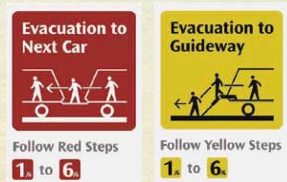
Figure 8: Red signage showing instruction for car-to-car evacuation, whereas the yellow signage showing instruction for direct evacuation to guideway
