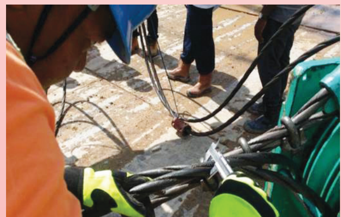
Figure 3: Safety Coordinator demonstrating the use of digital Vernier Calliper to check the diameter of wire rope
