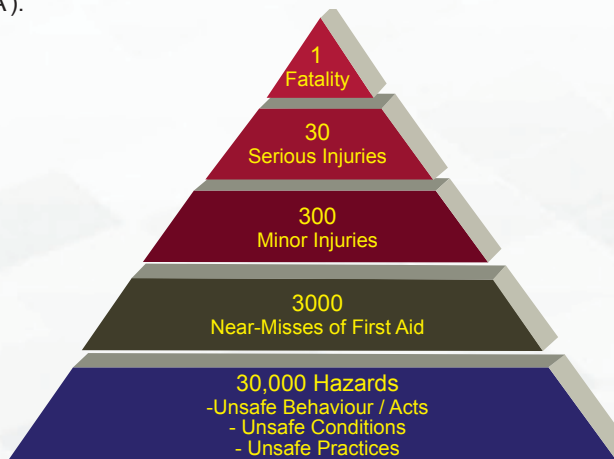
Figure 2: Typical Accident Pyramid (DuPont Model)
