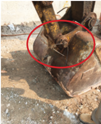
Figures 4: Non-original pin used to secure excavator bucket
