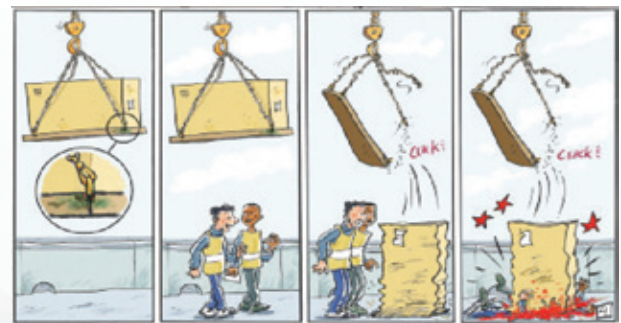
Unsafe condition ◦ Unsafe act ◦ Near miss ◦ Accident
