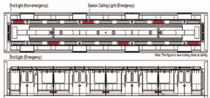
Figure 5: Train car emergency lighting location (in red)
