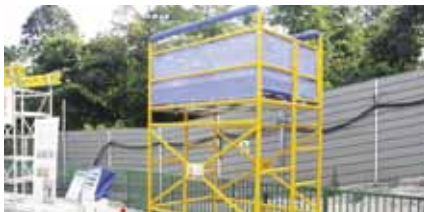
Figure 7: Mobile scaffold simulator
