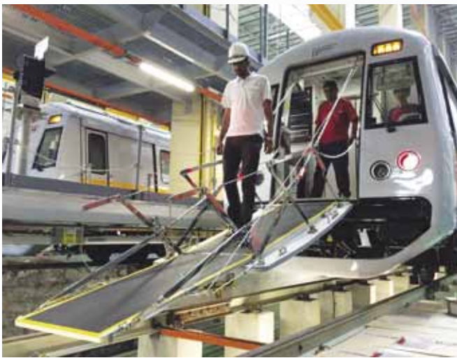
Figure 4: Detrainment door deployment test
