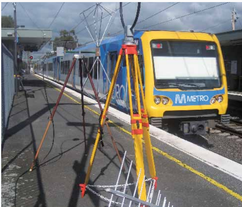
Figure 3: On-Site Train Emission Measurement
