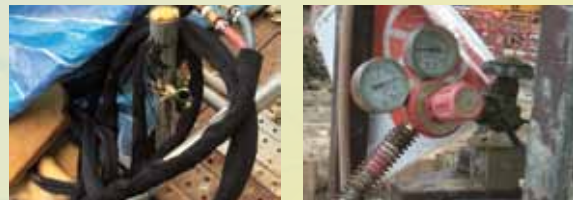
Figure 3: Engineering control to protect gas hoses
