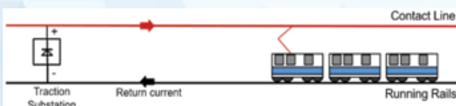
Figure 3: DC traction current flow for train operation
