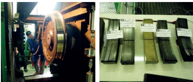
Figure 2: Dynamometer and brake blocks used in dynamometer test
