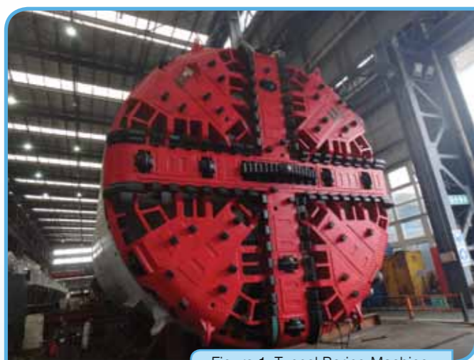
Figure 1: Tunnel Boring Machine
