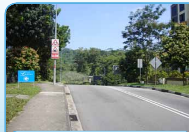
Figure 8: Warning signs provided to alert motorists of an upcoming roundabout junction after the crest of the vertical curve
