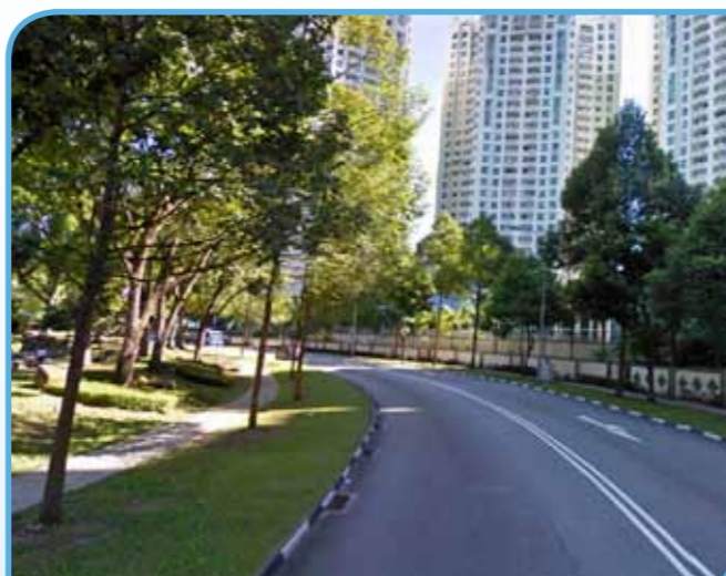
Figure 4: Trees planted away from the edge of the carriageway
