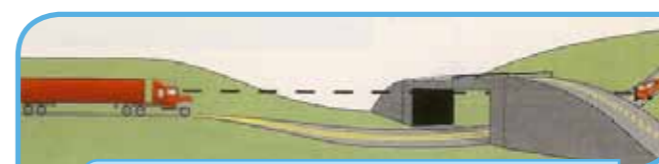
Figure 7: Visibility across the sag of a vertical curve
