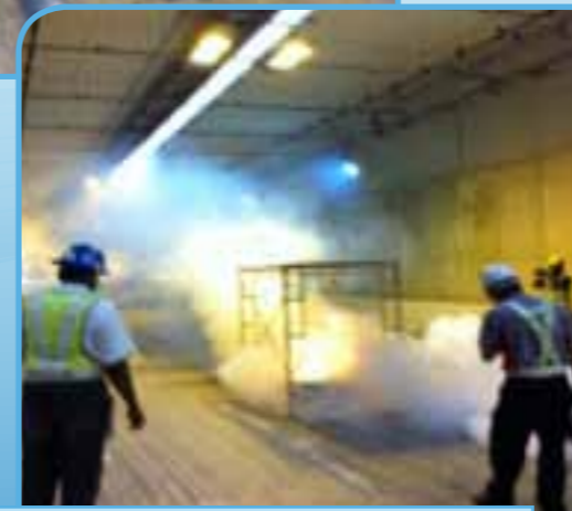
Figure 5: Use of fogging gun for smoke generation
