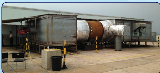
Figure 4: Factory Acceptance Test - High temperature test setup
