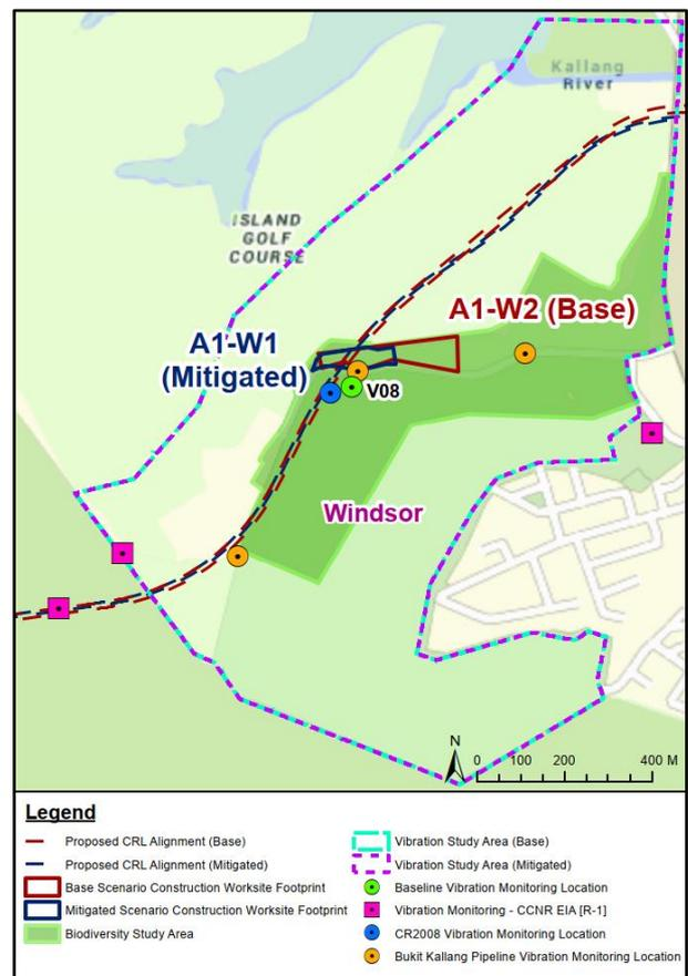
Figure 23: Vibration Baseline Monitoring at Windsor<sup>2</sup>
