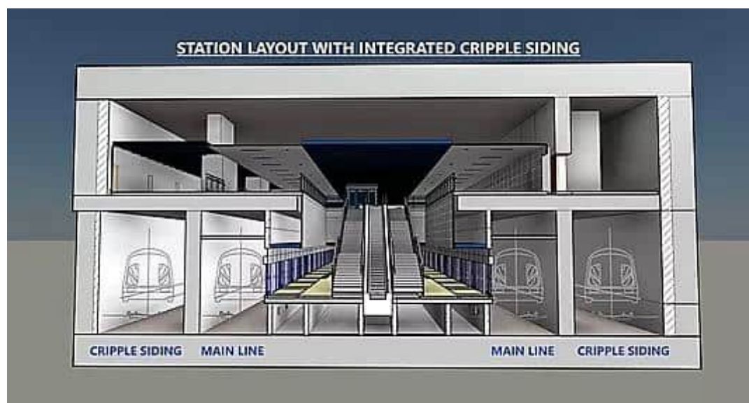
Figure 3-38 Example of Station Layout (Island Platform) with Integrated Cripple Sidings [W-36]
