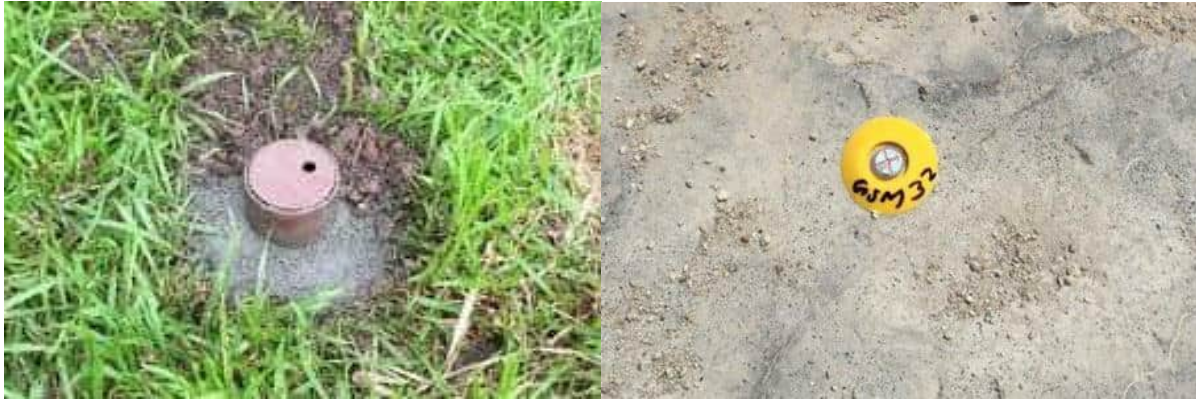
Figure 3-17 Example of Settlement Markers [W-6]
