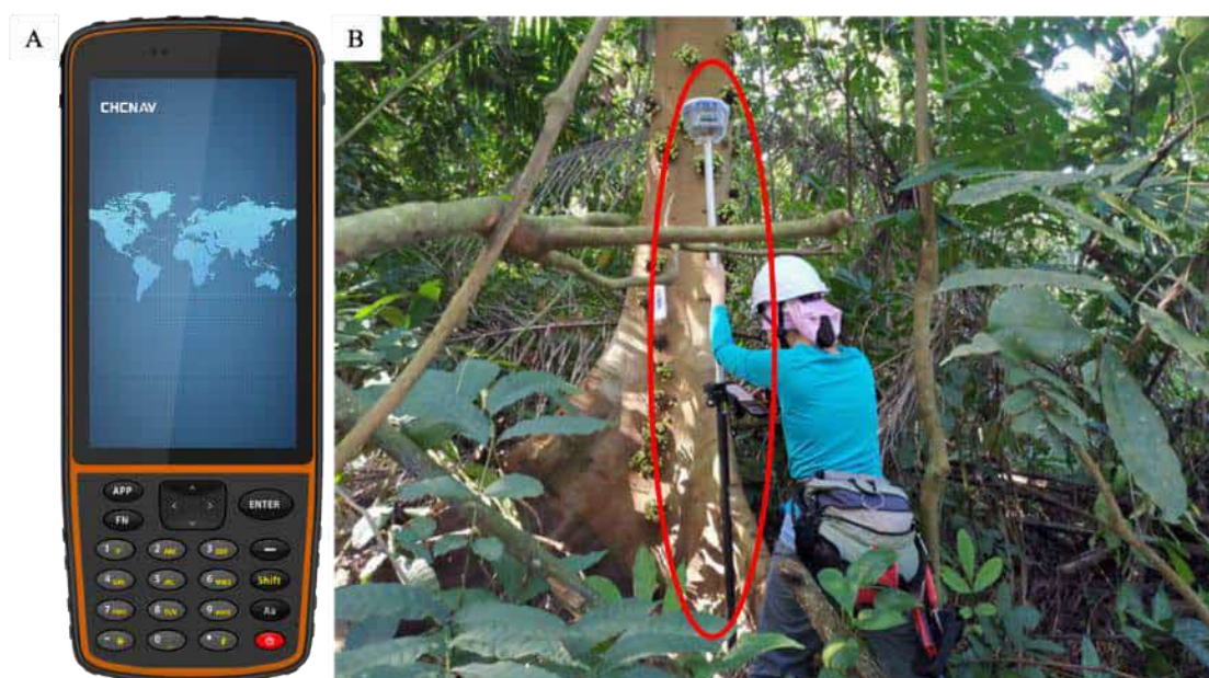
Figure 7-4 (A) CHC® Navigation HCE320 GNSS Data Controller (Source: Geo-matching.com); (B) How It is Used in the Field
