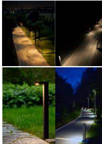
Figure 7-85 Low Level Bollards Directed Downwards and Shielded to Limit Lighting to Only the Area Intended
