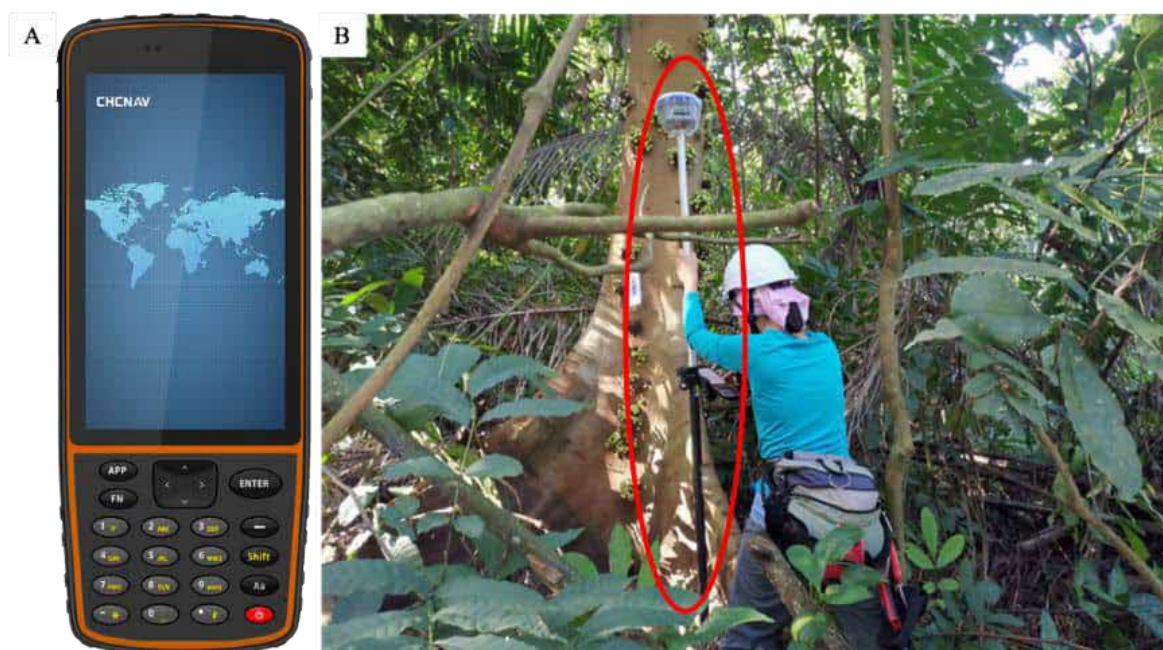
Figure 7-8 (A) CHC® Navigation HCE320 GNSS Data Controller (Source: Geo-matching.com); (B) How It is Used in the Field
