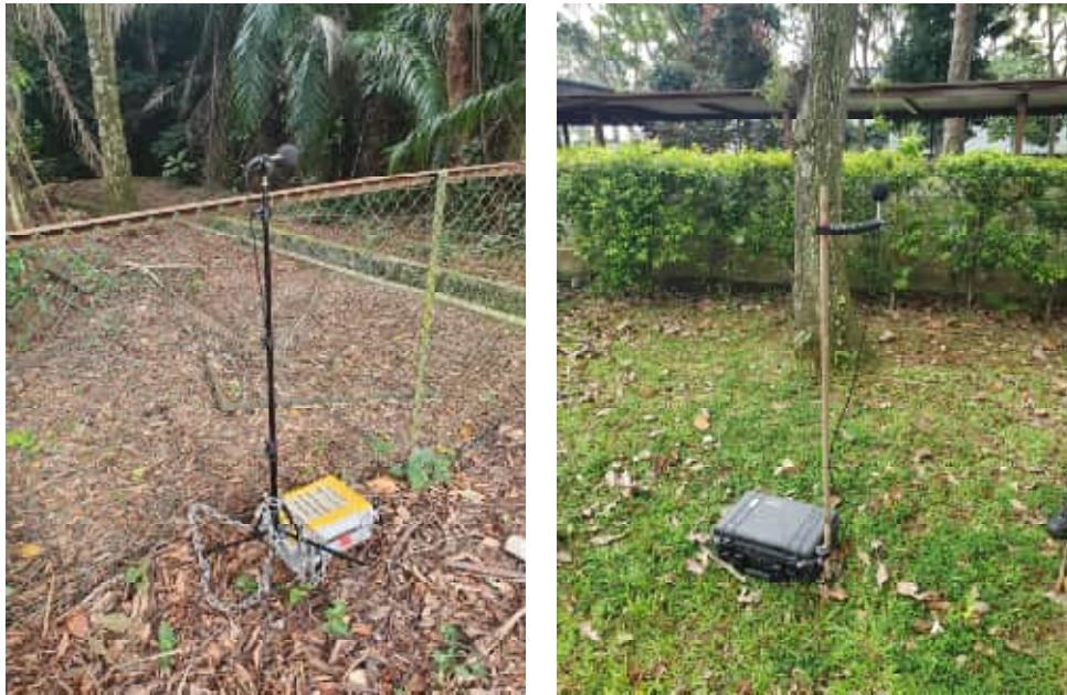
Figure 1 Airborne Noise Monitoring Setup
