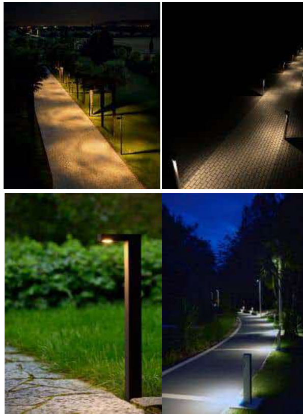
Figure 7-80 Low Level Bollards Directed Downwards and Shielded to Limit Lighting to Only the Area Intended
