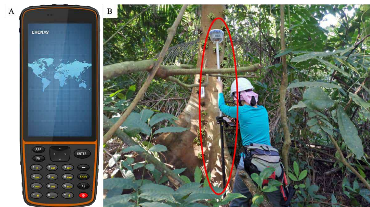
Figure 7-7 (A) CHC® Navigation HCE320 GNSS Data Controller (Source: Geo-matching.com); (B) How it is Used in the Field.
