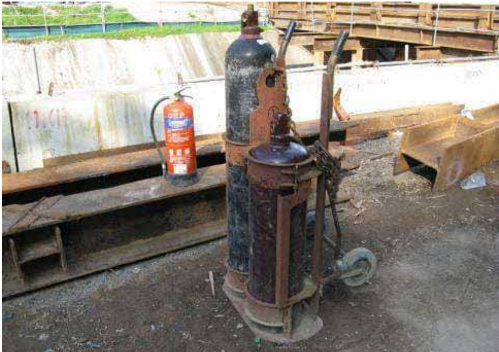
Gas cylinders secured in a cylinder trolley to prevent toppling
