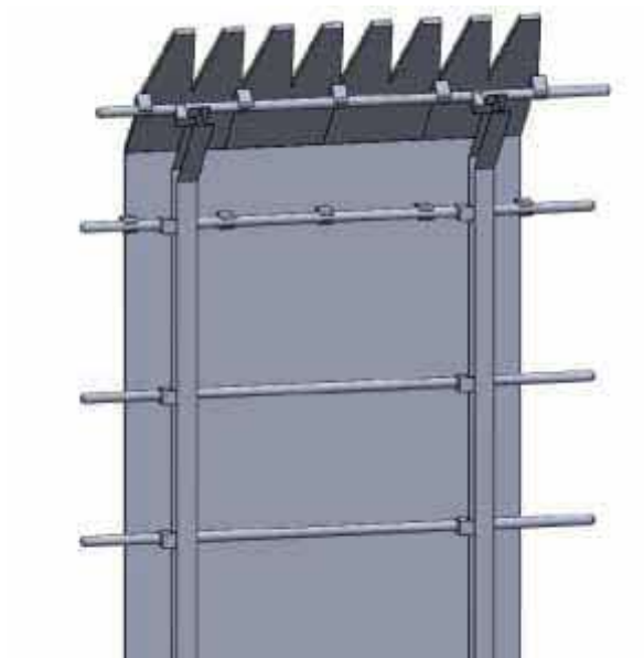
Indicative design of jagged edge flat-tip barrier
