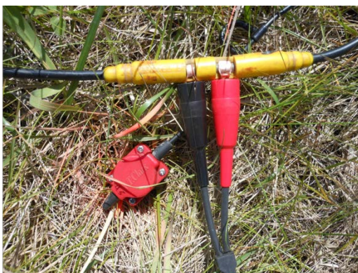
Geophone sensor and connection to cable (ARUP, 12.12.2014)
